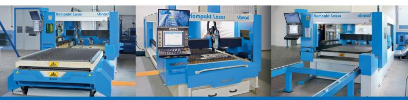
Vanad KOMPAKT Laser with two hydraulically exchangeable material grids and 2kW IPG laser source, installed in 2016 Vanad KOMPAKT Laser with a manually exchangeable material grid and 3kW IPG laser source, installed in 2017 Vanad KOMPAKT Laser with a motor-powered extendable material grid and 1kW IPG laser source, installed in 2017
