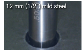
12 mm (1/2") hole without True Hole technology
