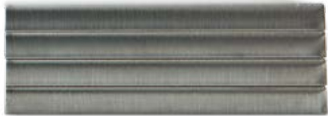
Range 2 cuts on 6 mm (1/4") mild steel
