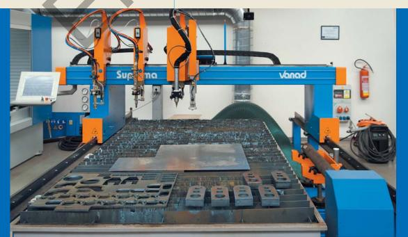
SUPREMA cutting station built in 2014. The CNC cutting machine is equipped with the Hypertherm Powermax 125 plasma system and oxy-fuel technology.
