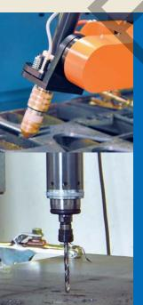
The 3D automatic plasma head extends the usage possibilities of the BLUESTER CNC machine
