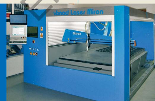
MIRON Laser is an efficient CNC cutting machine equipped with fiber laser, which effortlessly cuts metal and non-metal materials such as mica plates, HSS sheets, klingerit, mirelon, polyethylene foam, antivibration rubber sheets, cardboard, cork, brass, bronze, copper and tar paper.
