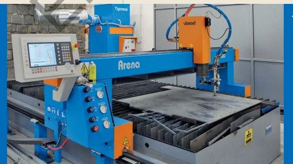
The ARENA CNC cutting machine with a touch panel and oxy-fuel torch. The oxy-fuel torch is equipped with IHT height control system. Tigemma exhaust and filter unit form a part of the station
